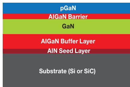
Figure 1.15 An additional GaN layer, doped with p-type impurities can be added to the heteroepitaxy process when producing an enhancement-mode device, as illustrated in Figure 1.10.
